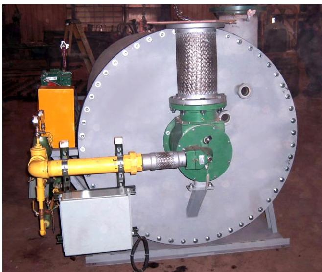
*ThermJet Burner mounted on limestone heater*
