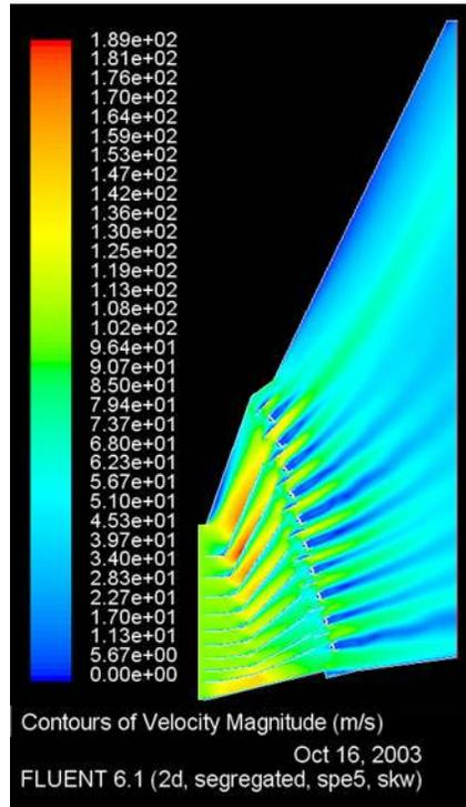
*CFD generated velocity contours before and after the addition of distribution plates illustrating improved flow distribution into the HRSG.*
