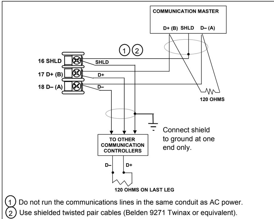
**Figure 2-15 RS-422/485 Communications Option Connections**
