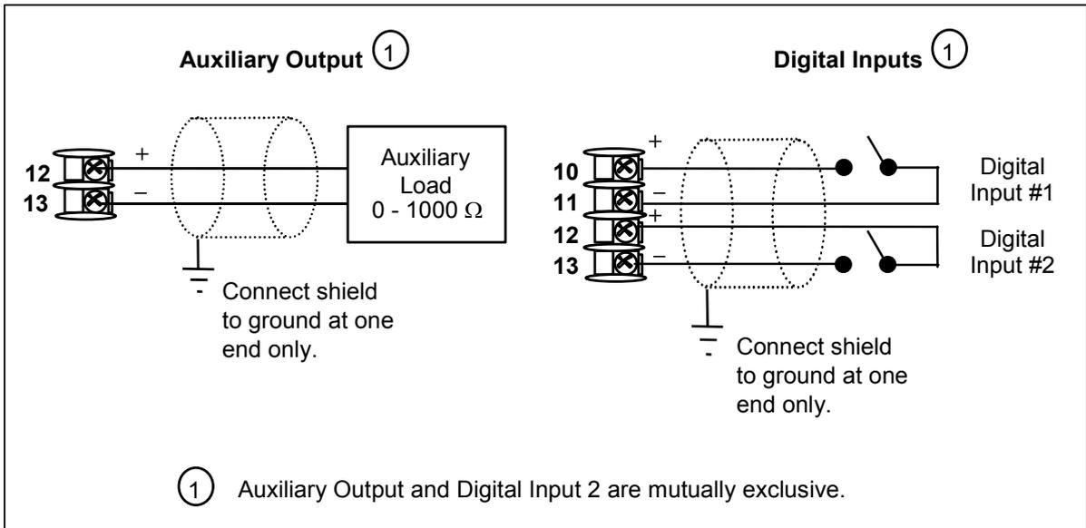
**Figure 2-17 Auxiliary Output and Digital Inputs Option Connections**
