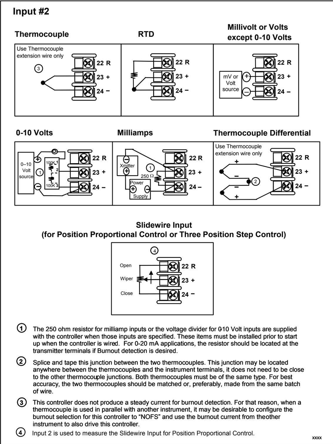
**Figure 2-7 Input 2 Connections**
