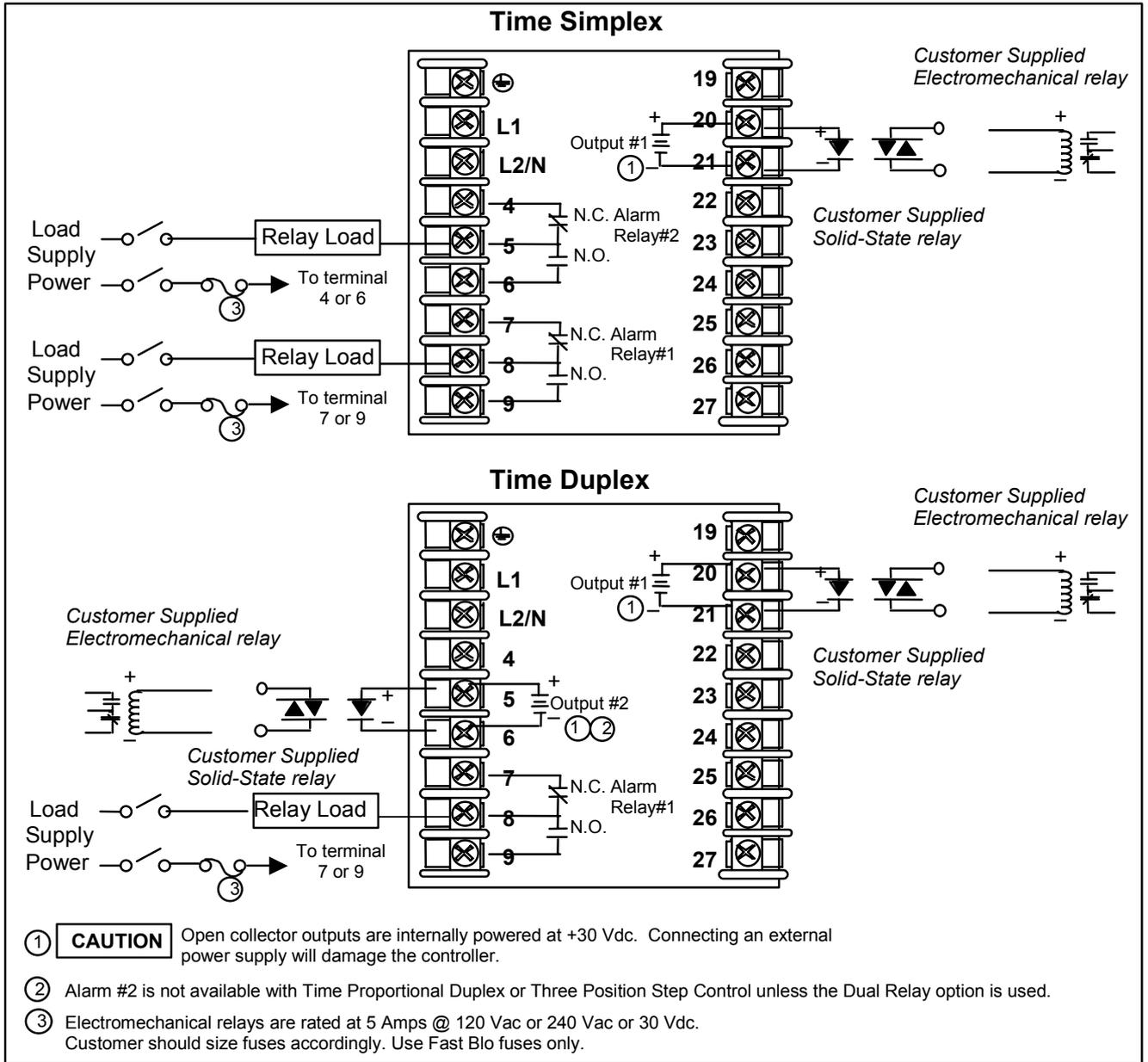
**Figure 2-10 Open Collector Output**
