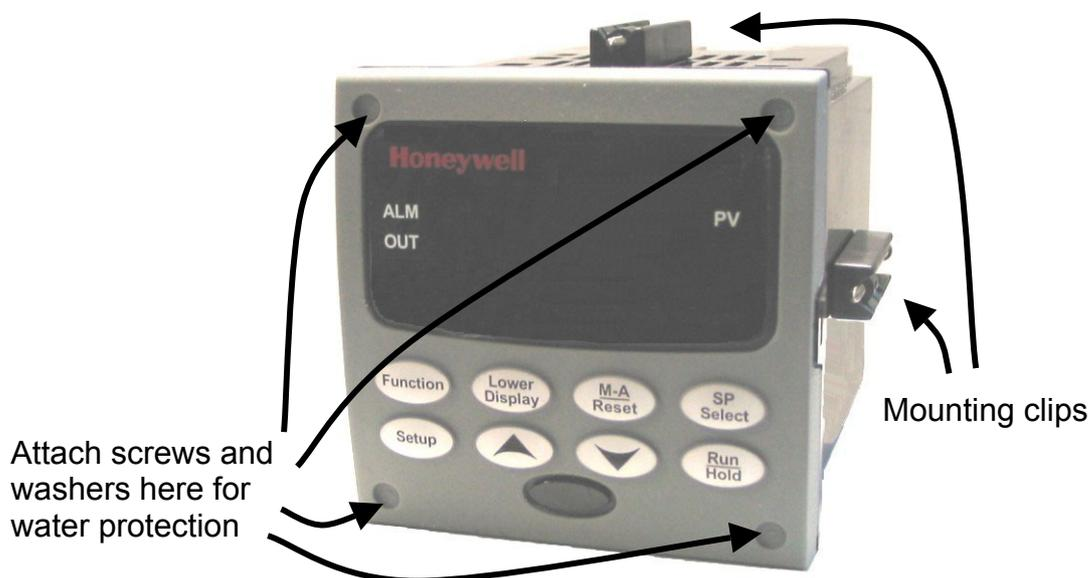
Figure 2-3 Mounting Methods
