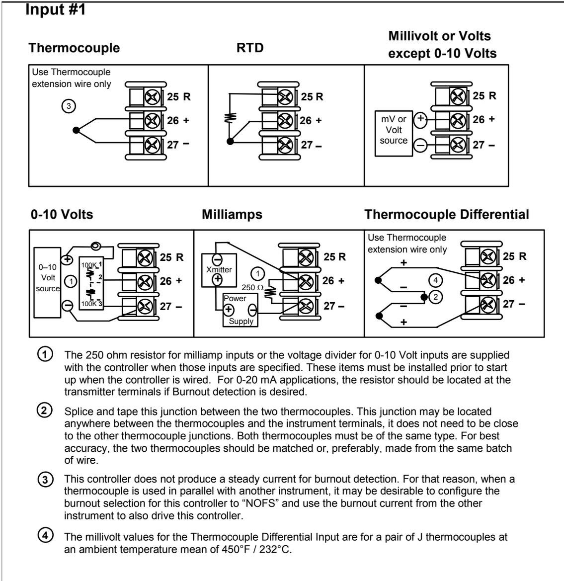
**Figure 2-6 Input 1 Connections**
