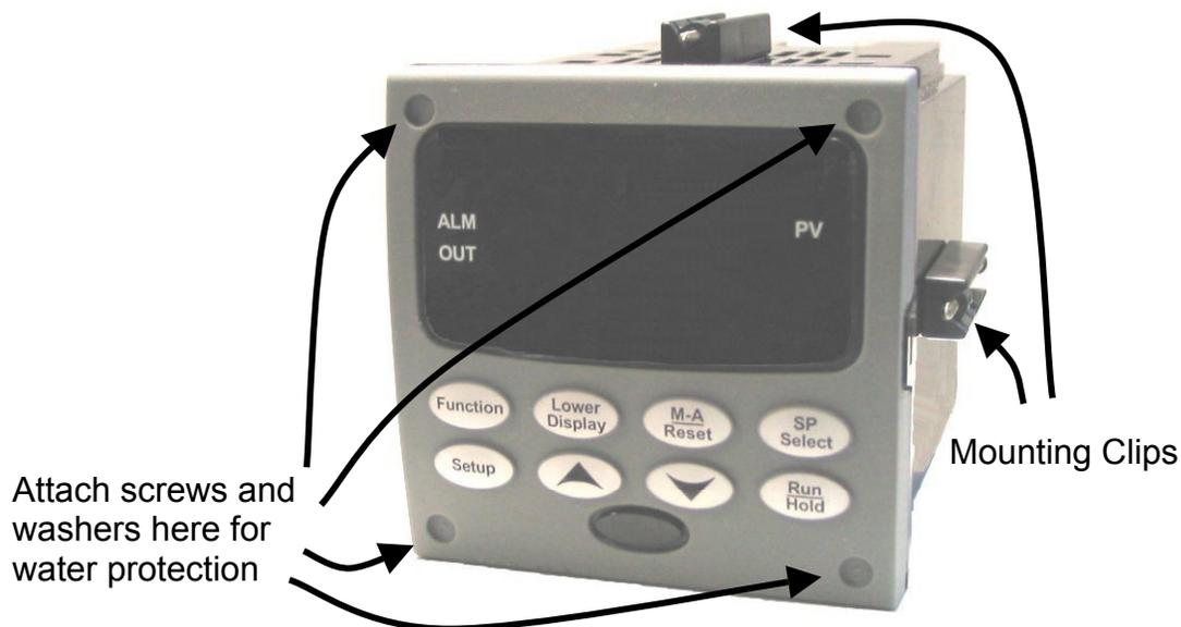
**Figure 2-3 Mounting Method**
