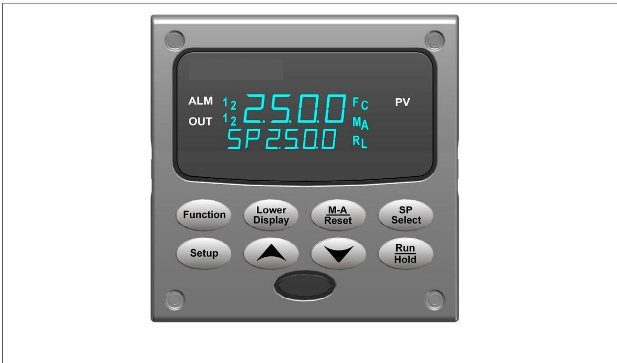
Figure 1-1 UDC2500 Operator Interface
