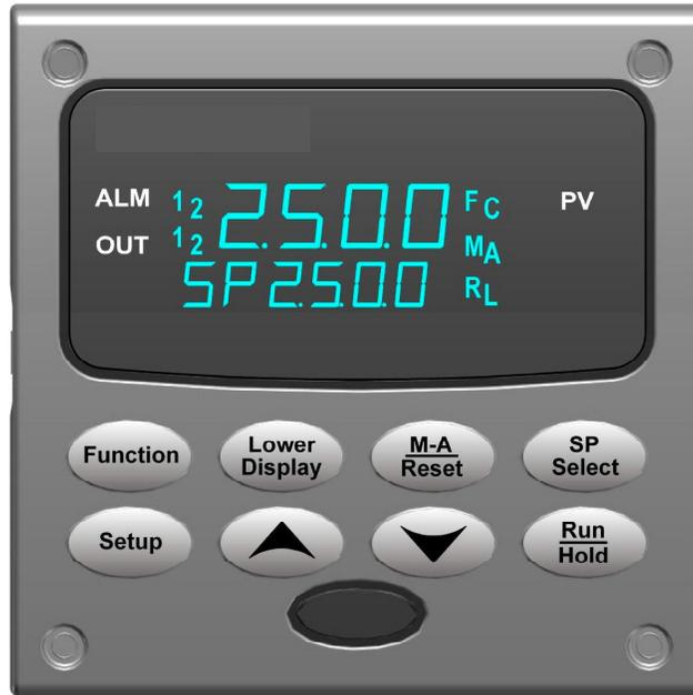
Figure 4-1 Operator Interface
