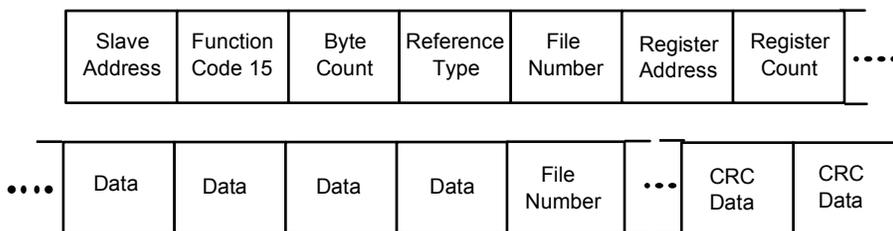
The register address is interpreted as the tag ID configuration number.
