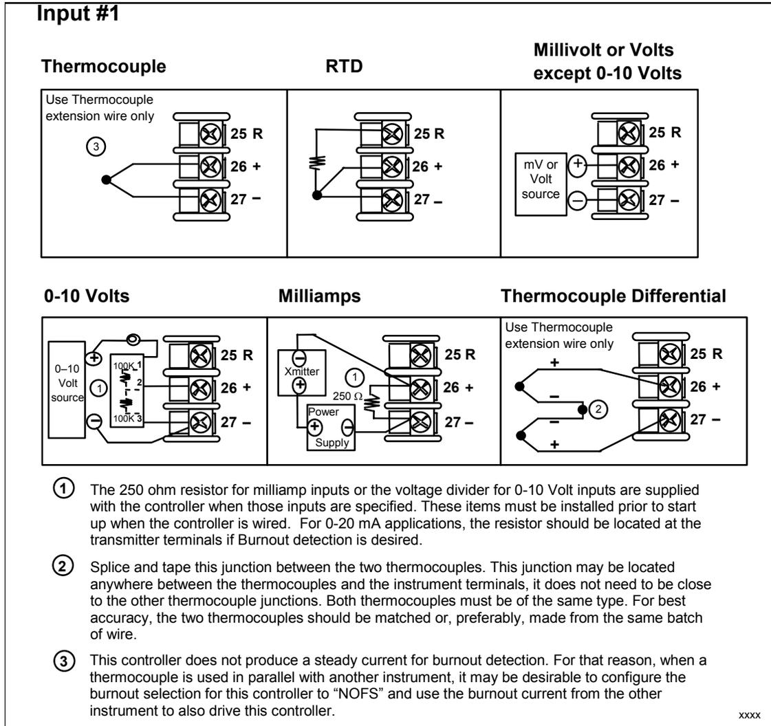
**Figure 2-6 Input 1 Connections**
