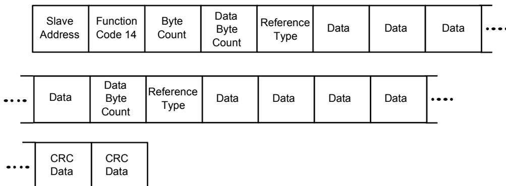
For Infrared Transactions, add three BOFs (C0hex) at the beginning of each message and one EOF (FFhex) at the end of each message.
