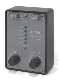
The Eclipse SimaFlame is a multifunctional tester that simulates flamerod or UV scanner flame signals to all major brand combustion safeguard controls. It also functions as a current loop checker. SimaFlame provides a variable 4-20mA output and can read 4-20mA inputs at five signal levels indicated by lights on the front face. These functions make this tool ideal for troubleshooting combustion control systems, including the temperature control loop.
