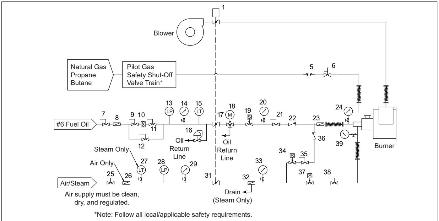
**Figure 3.7 - Schematic for #6 Fuel Oil**
