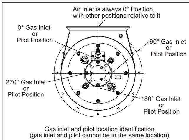
**Figure 3.1 - Gas Lance & Gas Pilot (Optional Positions)**
