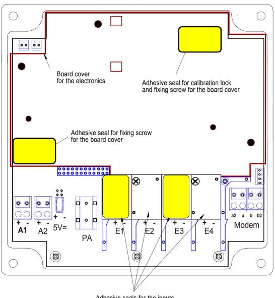
Adhesive seals for the inputs (only the inputs needed for legal calibration are sealed; e.g. here Inputs 1 and 3)
