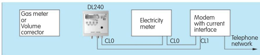
DL240 registration device for remote data transfer together with an electricity meter, connected to a telephone network via modem with CL interface
