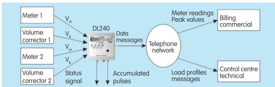
DL240 data collection device for a dual-stream gas metering system
