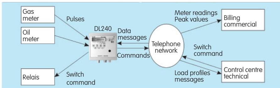
DL240 data collection device including remote-controlled digital output to switch from gas to oil
