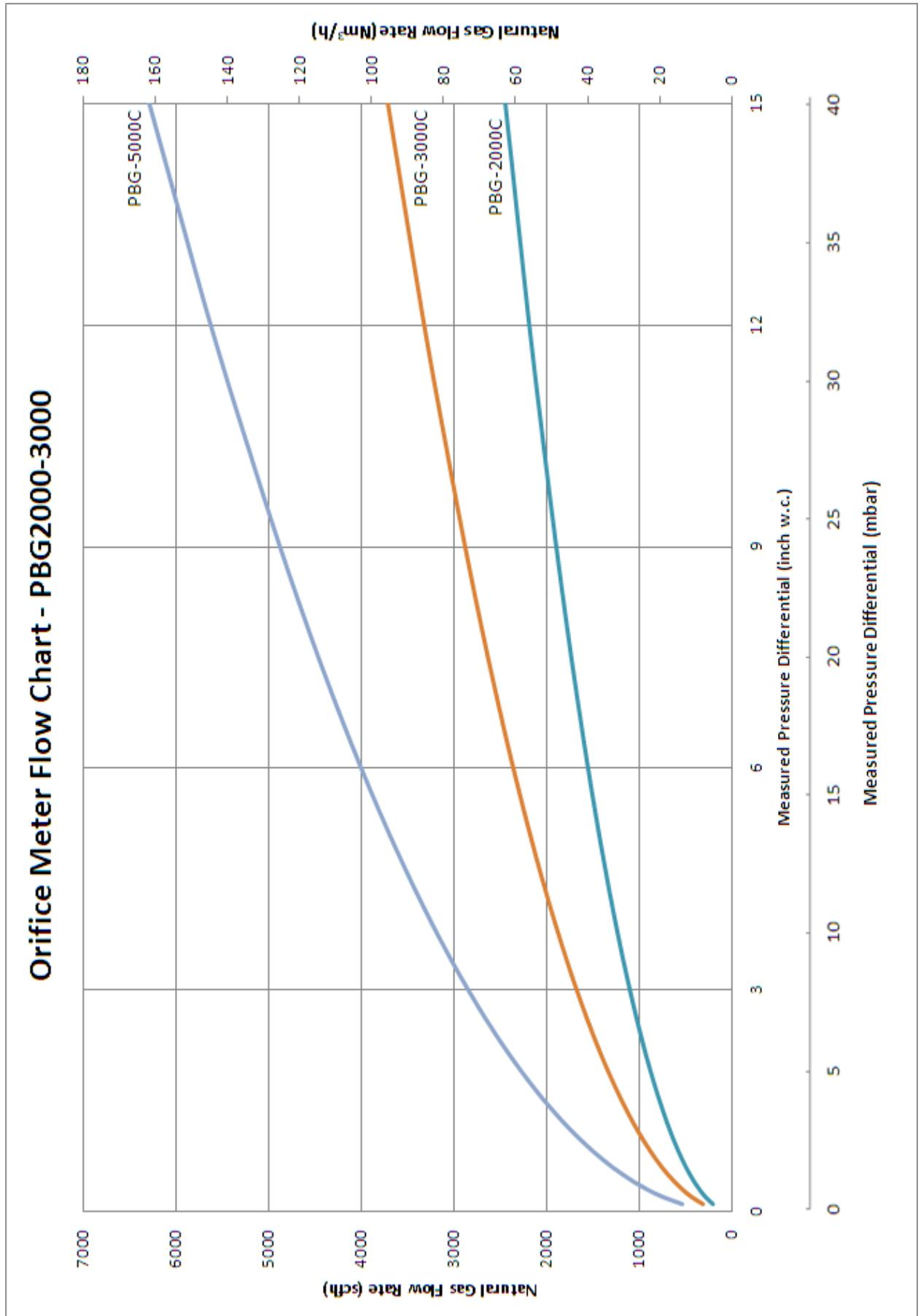
Figure 3. Natural Gas Pressure Drop vs. Flow across OMG
