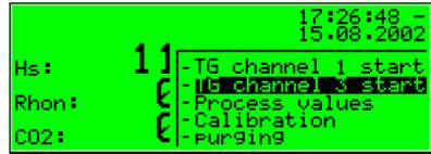
7. Now, the sensor system will be purged with test gas for about 2 minutes. Afterwards, the measurement begins. The measurement results are shown in the main display.
