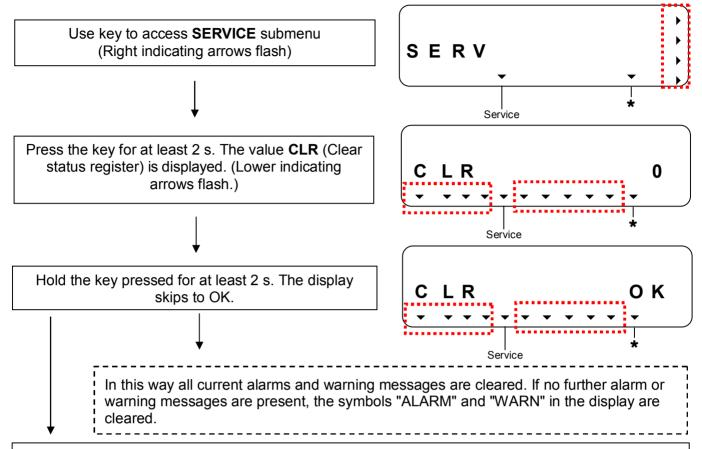
To **quit the submenu**, a value which cannot be edited is brought into the display. E.g. keep pressing the key until the **display test** is shown. The submenu is left by pressing the key for at least two seconds. The submenu is also left when the display switches off (after two minutes).
