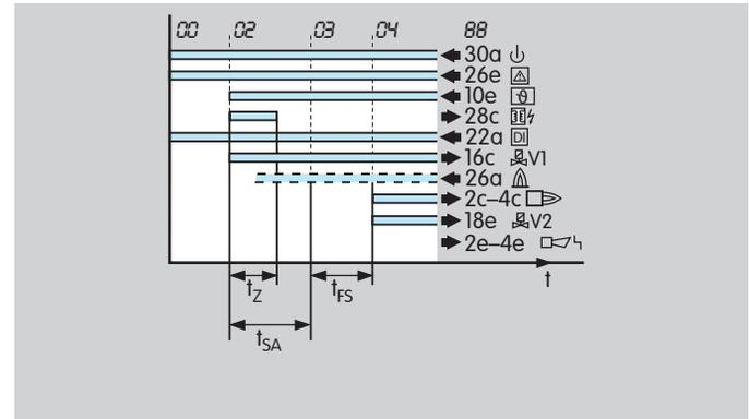
If the temperature in the furnace chamber drops below 750°C, the DI input must be disconnected from the electrical power supply and the furnace must be operated with the internal flame control system.
