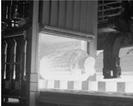
*Bogie hearth forging furnace
