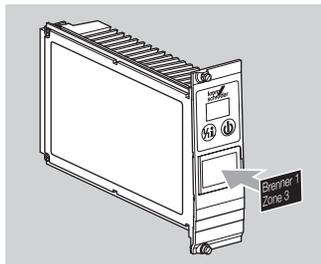
For printing with laser printers, plotters or engraving machines, 27 × 18 mm or 28 × 17.5 mm.
