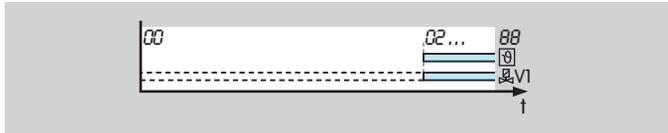
Parameter 15 = 1: The flame simulation check is conducted provided no start-up signal ( $\vartheta$ ) is applied (during the so-called start-up position/standby). This allows fast start-up of the burner since there is no waiting time  $t_W$ .
