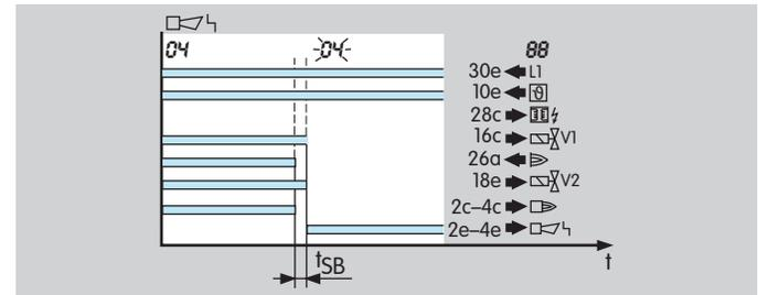
If the flame fails during operation, the valve outputs are disconnected within the safety time  $t_{SB}$ .
