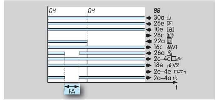
If the flame fails during high temperature operation, the ready contact is opened for the duration of the flame failure.
