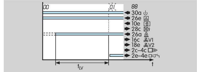
An extraneous signal is an incorrect signal which is detected as a flame signal out of sequence. If the PFU 760 notices such an extraneous signal during the flame simulation check, it starts the flame simulation delay time  $t_{LV}$ . If the extraneous signal is discontinued during this period, the burner can start up. Otherwise, a fault lock-out occurs.  $\square 01$  blinks on the display.
