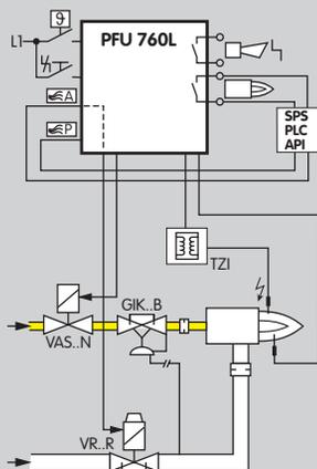
Parameter 30 = 0: The air valve opens if it is activated externally by input 10a.
