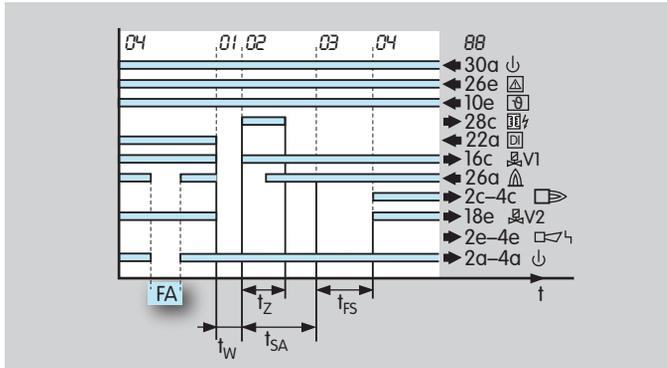
If the flame fails during high temperature operation, the ready contact opens for the duration of the flame failure (FA).
