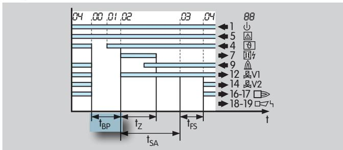
An immediate restart of the main burner after a controlled shut-down, a start-up attempt, restart, cooling or purging is prevented by the pause time. The pause time starts when the air valve is switched off. If a start-up signal ( $\ominus$ ) is applied before expiry of this time, the start-up is delayed until the end of the pause time.
