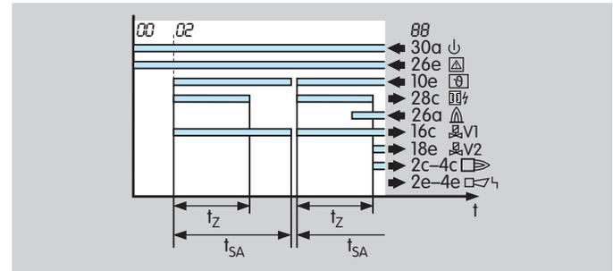
If several start-up attempts are set and if the PFU detects a flame failure during start-up, it closes valve V1 after the safety time  $t_{SA}$  has expired and attempts to start up again. After the last programmed start-up attempt has been completed, the burner control unit conducts a fault lock-out. The display blinks and shows the cause of the fault.
