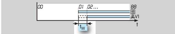
Parameter 15 = 0: The flame simulation check is conducted after applying the start-up signal ( $\vartheta$ ) during the waiting time  $t_W$ .
