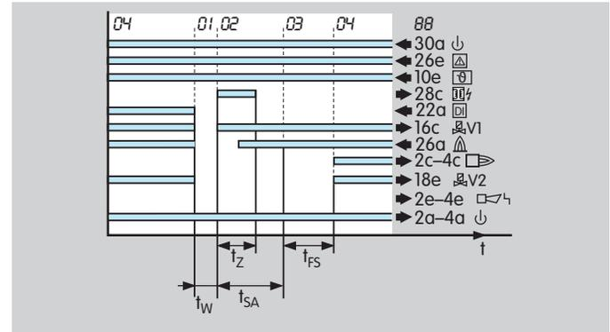
When High temperature mode is ended, the PFU switches off the burner and restarts with flame simulation check (recommended in the case of UV control with UVS).
