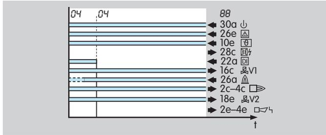
When High temperature mode is ended, the burner remains in operation and the PFU performs flame control again (recommended in the case of ionization control or UV control with UVD).
