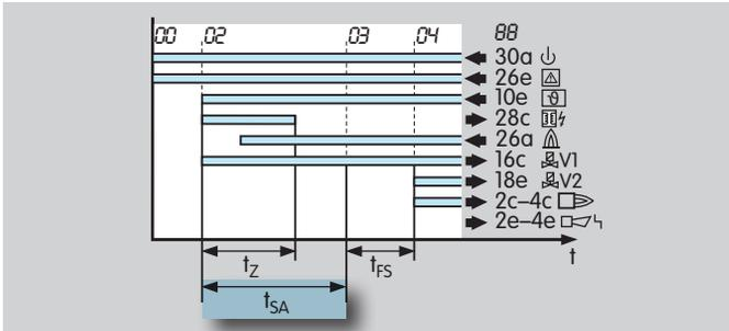
Safety time on start-up  $t_{SA}$  for the burner.
