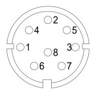
1: Output 1 - (A1-) 2: Output 1 + (A1+) 3: Output 3 - (A3-) 4: Output 3 + (A3+) 5: Output 2 - (A2-) 6: Output 2 + (A2+) 7: Output 4 - (A4-) 8: Output 4 + (A4+)
