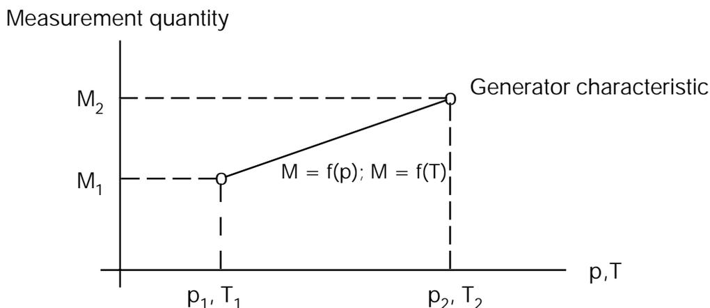
The characteristics for the pressure and temperature sensors are approximately linear and are determined by two points. For recording a characteristic for the pressure range two pressure values are entered under the reference code P27 one after the other after these values actually appear on the pressure generator.
