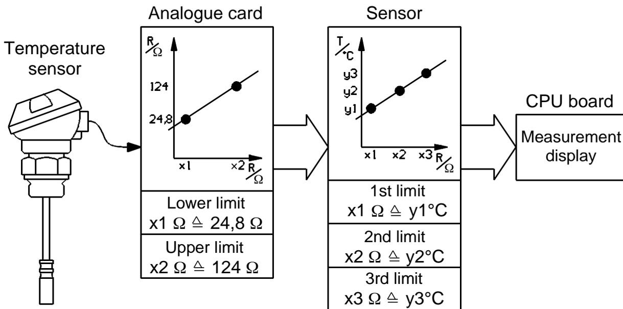
**Figure: Correction of the temperature sensor characteristic.**
