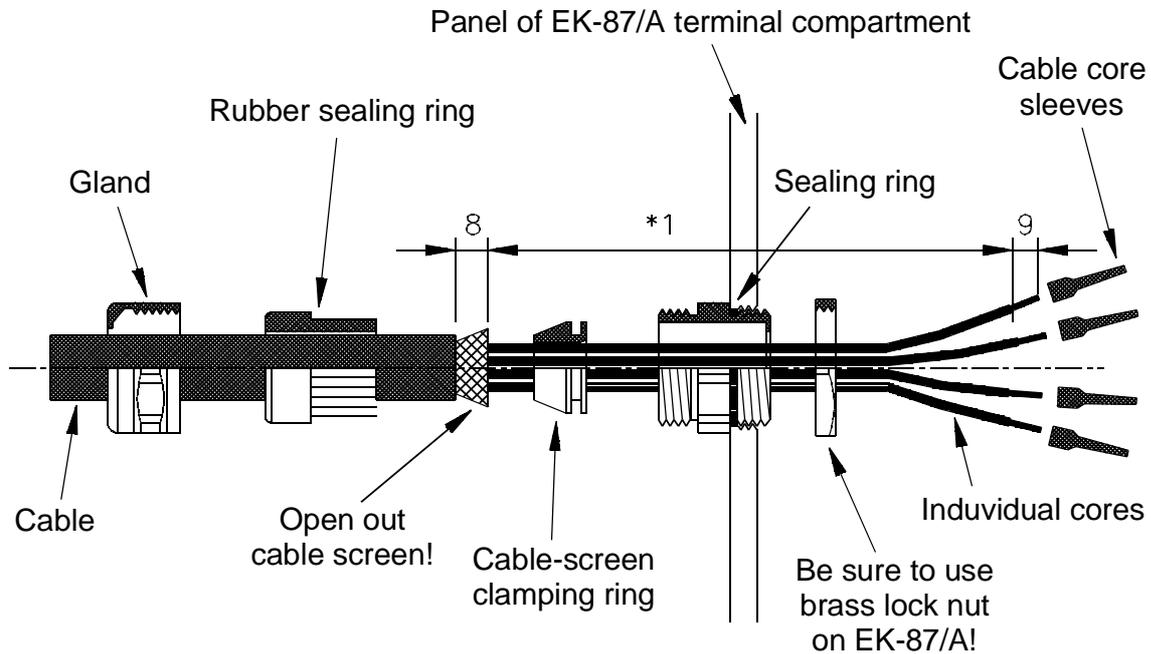
\*1: Length of single cores: 50 - 100 mm depending on connection!
