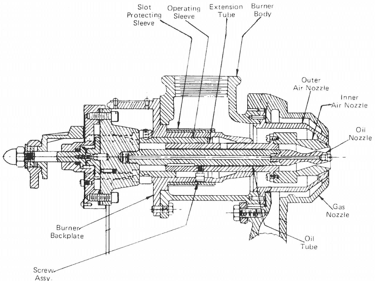
**Figure 5. Cutaway Showing Burner Components**
