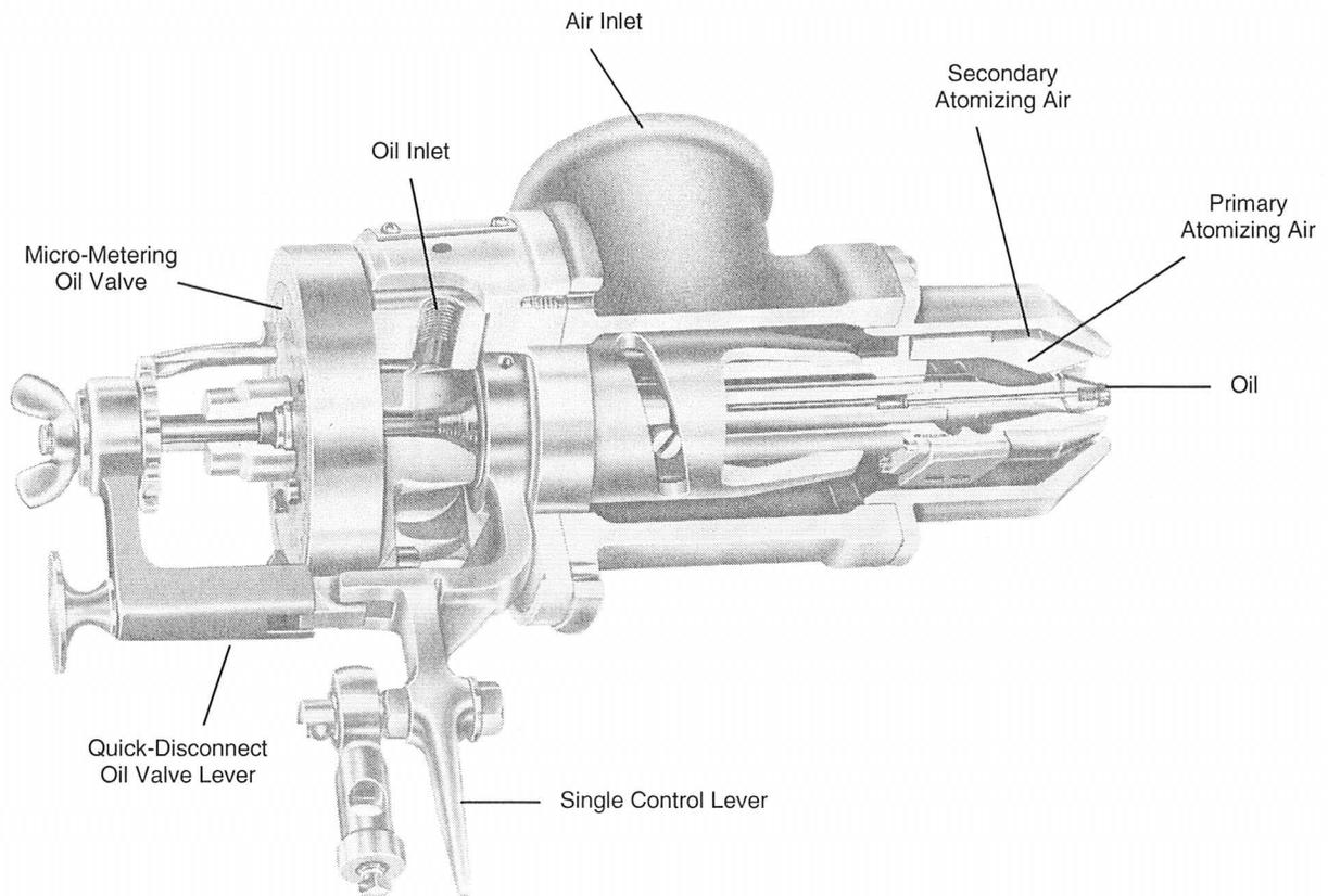
**Figure 6. Sectional View Of Burner**
