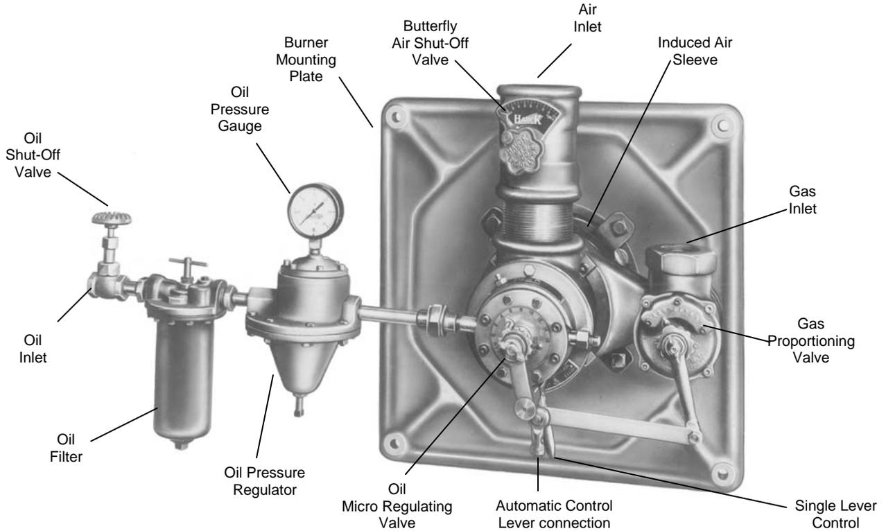
**Figure 1. Typical 780 Series Burner Arrangement Showing Components.
