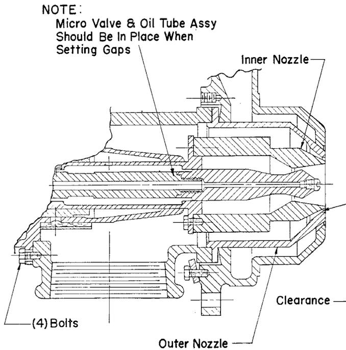
Figure 2. Schematic representation depicting the inner and outer nozzles.
