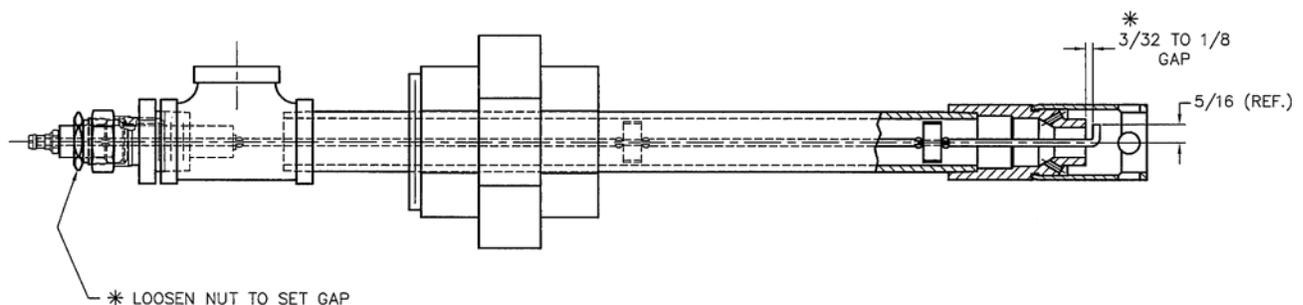
**Figure 4. Replacement Electrode Bending Details**
