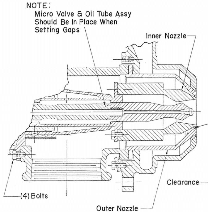
Figure 8. Schematic Representation Depicting The Inner and Outer
