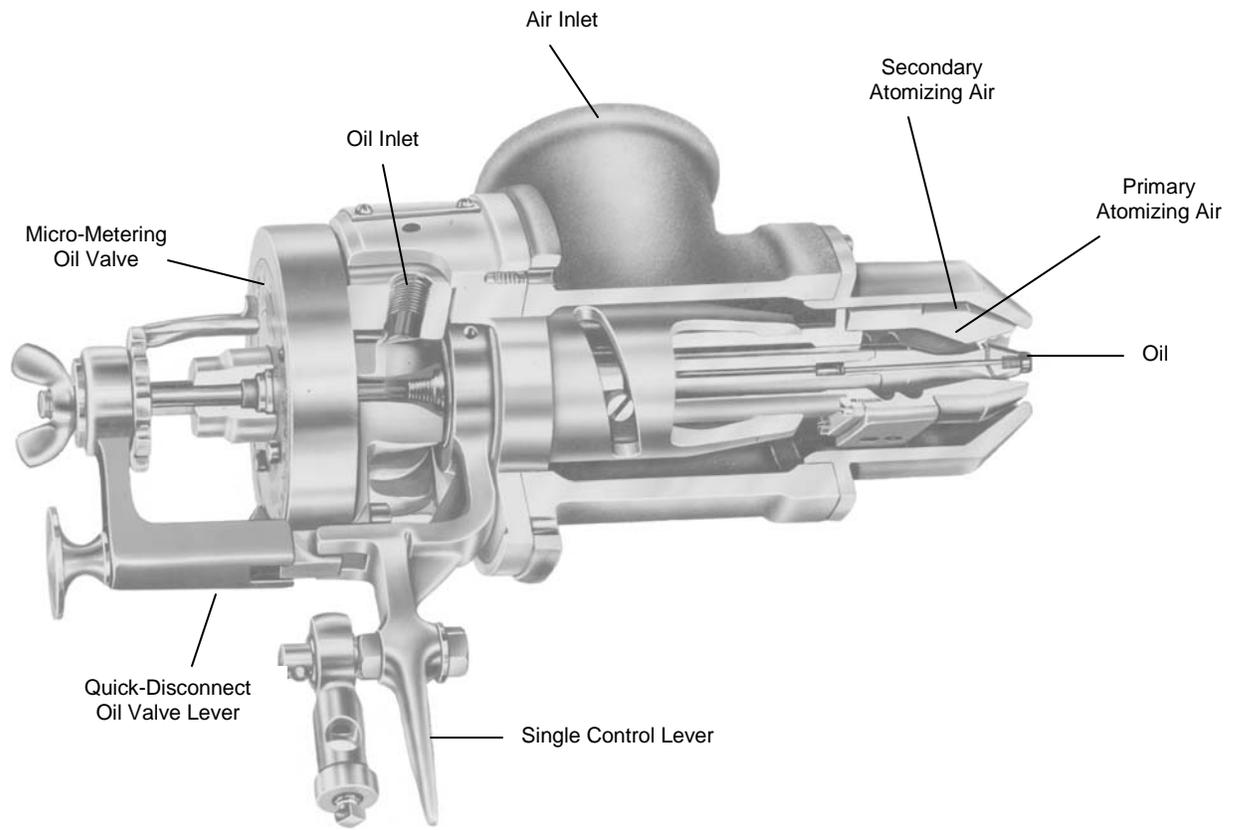
**Figure 5. Sectional View Of Hauck Self Proportioning Oil Burner**
