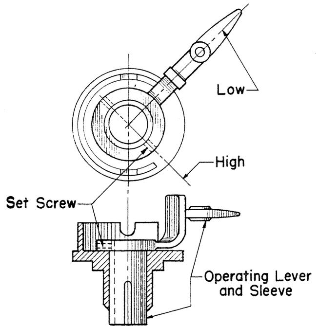
Figure 1. Drawing of the air nozzle control lever showing the set screw locations.
