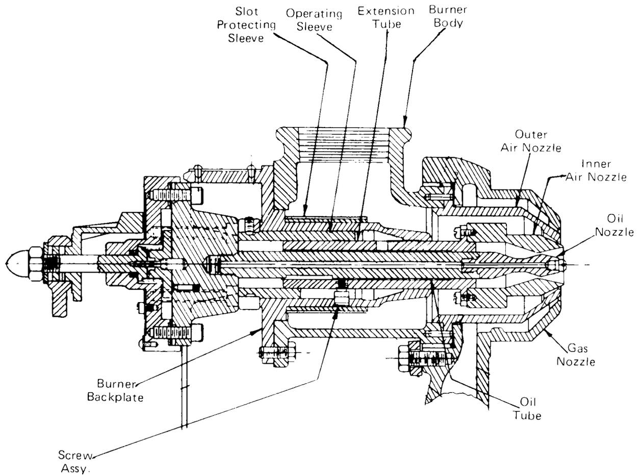
**Figure 4. Cutaway View Of The 780 Seires Burner Assembly Showing The Individual Components.**
