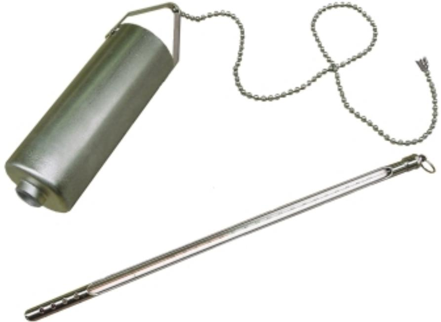
Hauck's Oil Viscometer Kit provides an easy, convenient and inexpensive way to rapidly determine the temperature to which oil should be heated to arrive at the proper viscosity for atomization. Kit includes viscometer and 0 - 300 °F scaled armor-cased thermometer.
