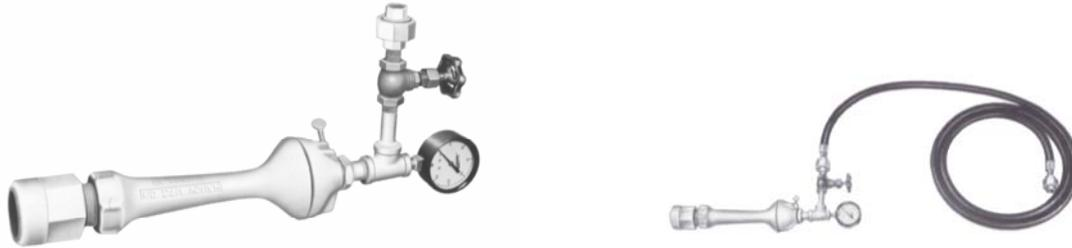
The Hauck "Ratio" Gas Torch combines a "Retain-A-Flame nozzle with an inspirator to produce a multi-purpose torch designed for use where gas pressures from 10 to 30 psig are available. The inspirator assists in maintaining the proper air-gas ratio under all operating conditions. This torch is designed for rugged duty in open air applications.
