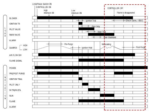
Fig 5b. Normal operation: NO-POST-PURGE configuration.
