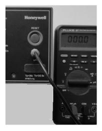
Fig. 4-3: Measuring flame signal with multi meter (µA range selection) using a jack plug.
