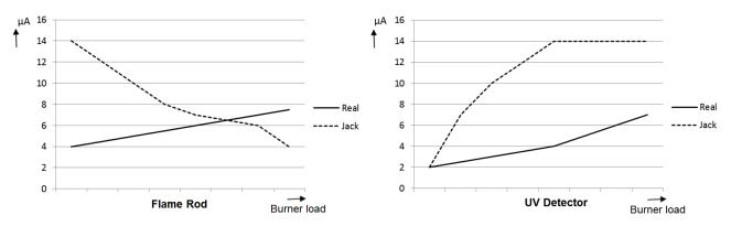
Fig. 4-2: Real flame current versus reading on frontal jack plug.
