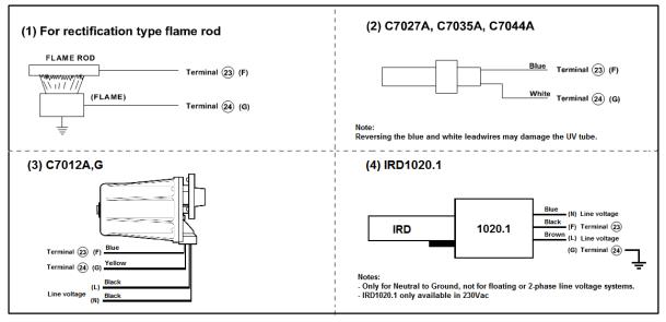
Fig. 4-1: Wiring a flame detector
