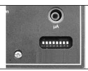
Note for DIP switches: on = upwards off = downwards
