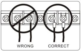
Fig. 2-1: Wiring the sub base terminals
