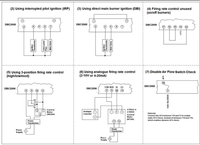
Fig. 3-3: More examples of wiring to external equipment
