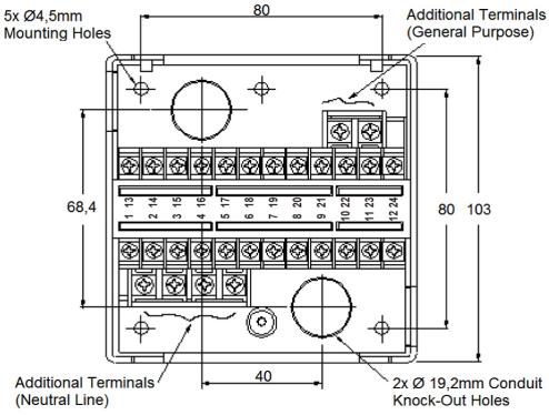
Fig. 2: Mounting dimensions of sub-base and terminal layout
