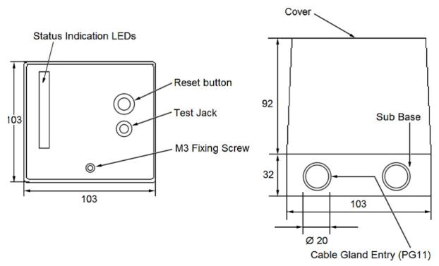
Fig. 1: External Dimensions (in mm)
