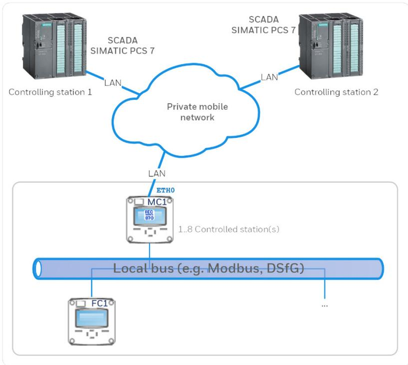
Fig. 2-1: Data communication via IEC protocol – example
