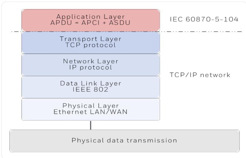
Fig. 2-1: The 5 layers of the IEC 60870-5-104 protocol
