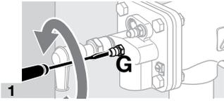
1 → Loosen the screw 2 turns.
