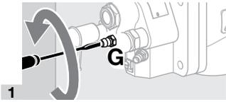
1 → Loosen the screw 2 turns.
