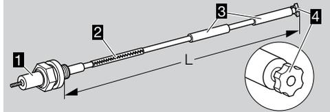
4 If the star 4 or insulator 3 is damaged, replace the electrode.
