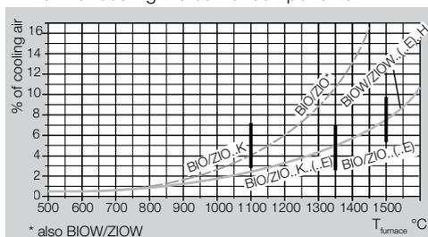
→ Diagram: the cooling air percentage specified in the diagram refers to the operating flow rate for air.
