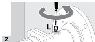
→ Loosen the screw 2 turns.
