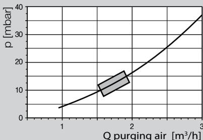
→ A purge air volume of approx. 1.5 to 2 m³/h per electrode is recommended.
