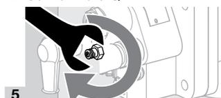
→ Tighten the lock nut. Do not alter the flow rate setting!
