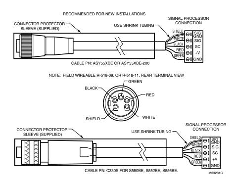
Fig. 2. Wiring connections for S550BE, S552BE, and S556BE viewing heads.
