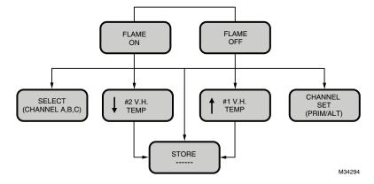
Fig. 11. Flowchart 4: Flame On / Flame Off.
