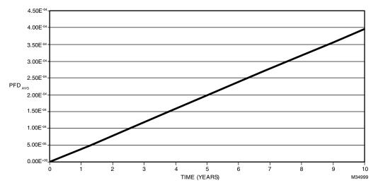
Fig. 12. P531 AC PFD<sub>AVG</sub> vs Time.
