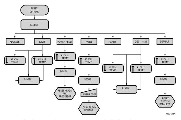
Fig. 10. Flowchart 3: Option Menu - System-wide Configuration Parameters.
