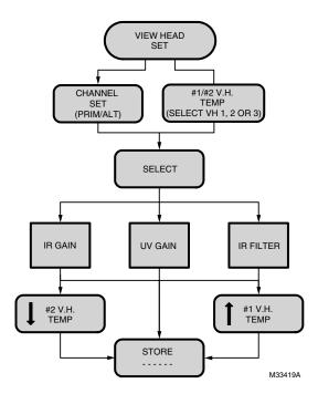
Fig. 8. Flowchart 1: Viewing Head Set, Channel Set and Option.
