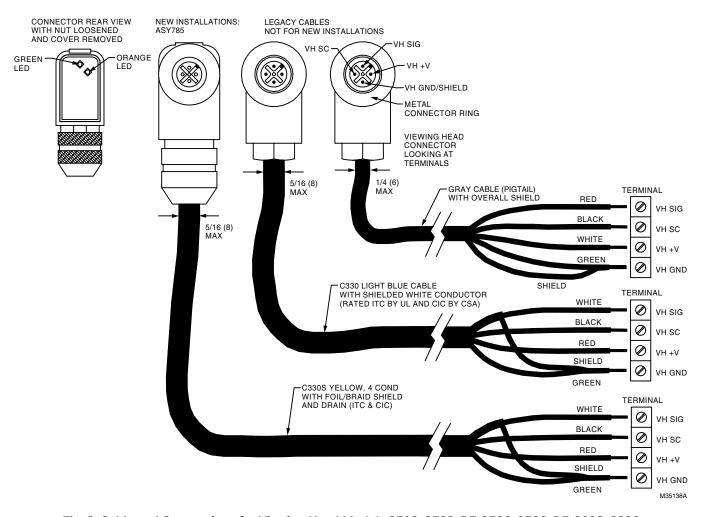
Fig. 3. Cable and Connections for Viewing Head Models S702, S702-PF, S706, S706-PF, S802, S806.
