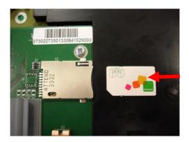
Insert the SIM card into the card slot until the spring resistance has been overcome (click!) and the card engages.
