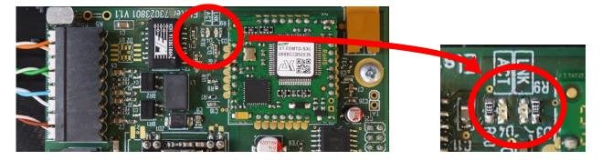
If the LEDs do not flash, either the module is not active (possible cause: the time window is still open) or there is a fault in the wiring.
