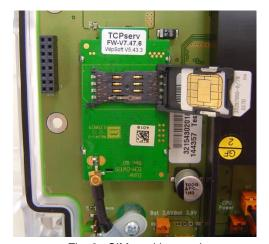
Fig. 8: SIM card inserted
