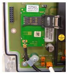
Fig. 7: Open SIM card slot
