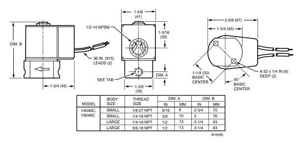
Fig. 2. V4046C, V8046C approximate dimensions in in. (mm).
