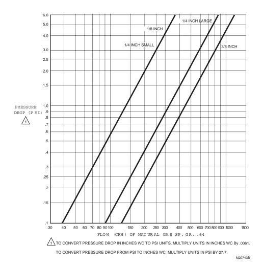
Fig. 1. Pressure drop (psi) vs.flow capacity (cfh) on V4046C, V8046C gas valves only.
