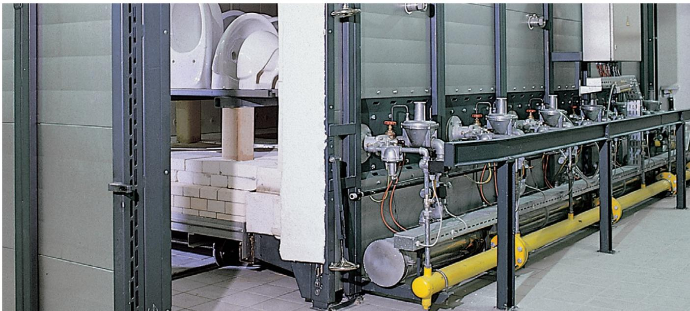
*Intermittent shuttle kiln, works photograph Eisenmann*
