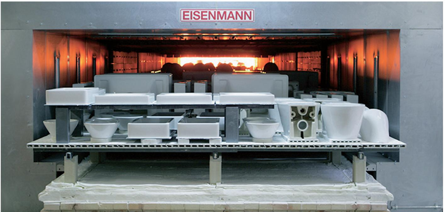
Intermittent shuttle kiln, works photograph Eisenmann
