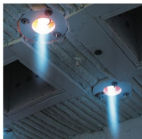
Overhead firing with BIC burners
