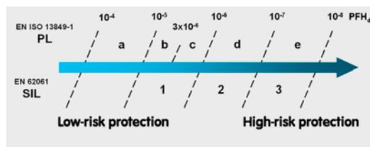
in this area of application – such as Safety Integrity Level (SIL) and Performance Level (PL) classification. Comprehensive risk analyses, which are the best possible way of identifying any potential risks, are at the heart of these considerations. The precisely harmonized measures of the individual safety functions for minimizing risks are then based on these.
