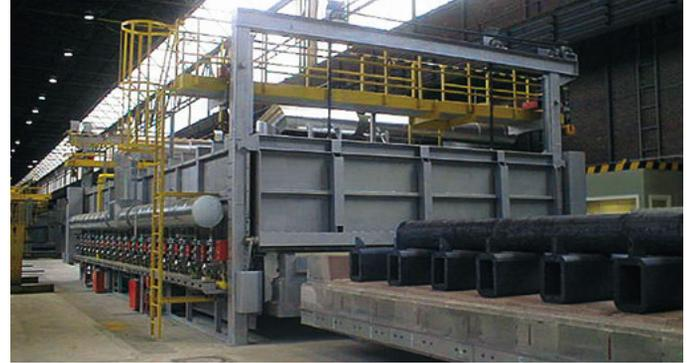
*Metallurgical industry: bogie hearth furnace*
