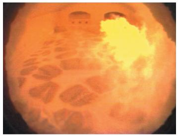
Internal view of regenerative glass furnace. (Photo was made from a still frame of a CCTV video)
