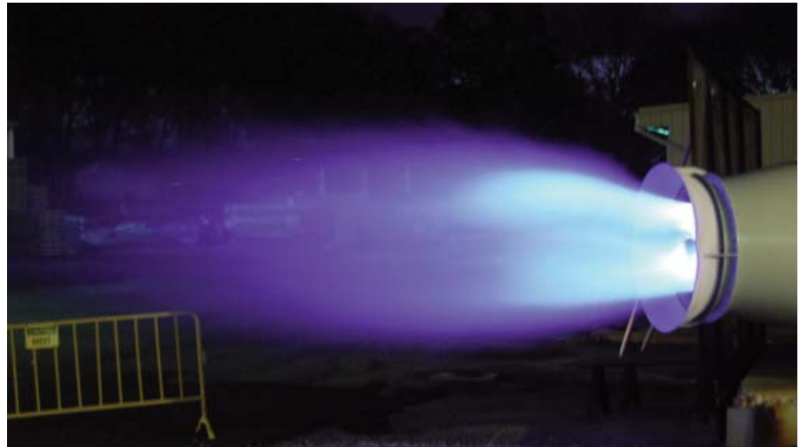
NovaStar NS150 firing natural gas at 140 MMBtu/hr
