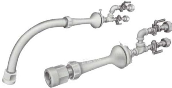
The Hauck “Booster” Torch combines a “Retain-A-Flame nozzle with a booster to produce a multi-purpose torch designed for use where low pressure gas and compressed air (ranging from 30 to 120 psig) are available. The booster assists in maintaining the proper air-gas ratio under all operating conditions. This torch is designed for rugged duty in open air applications.
