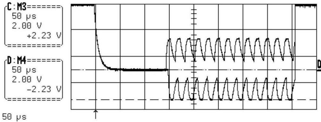
This example shows both a positive voltage and a negative voltage burst example in the same Chart.
