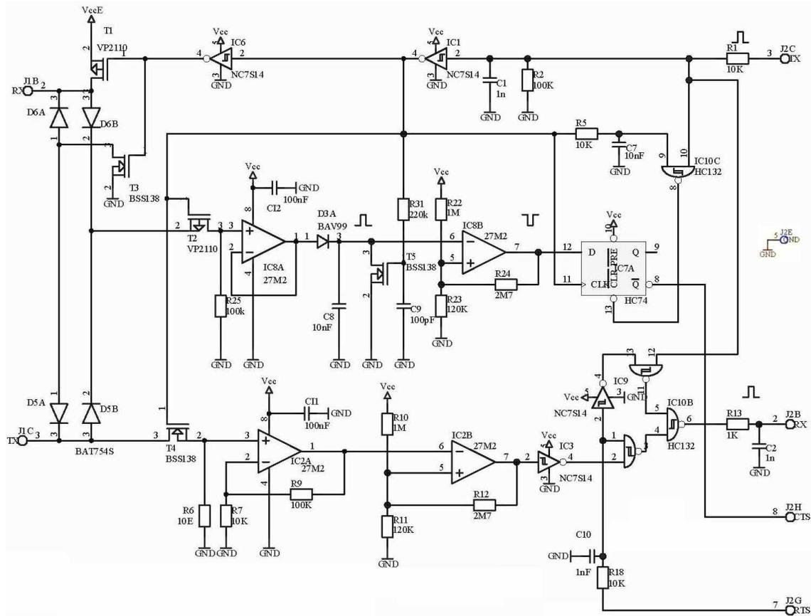
This example shows how a meter can be connected to a RS232 interface. To read the Standard SCR Protocol, the transmission unit with the RS232 simply switches RTS to high and Power on (not shown). To read the synchronous protocol, the transmission unit clocks its data output e.g. by sending 'p' with a baudrate of e.g. 19200 baud and checks its CTS input for incoming bits.
