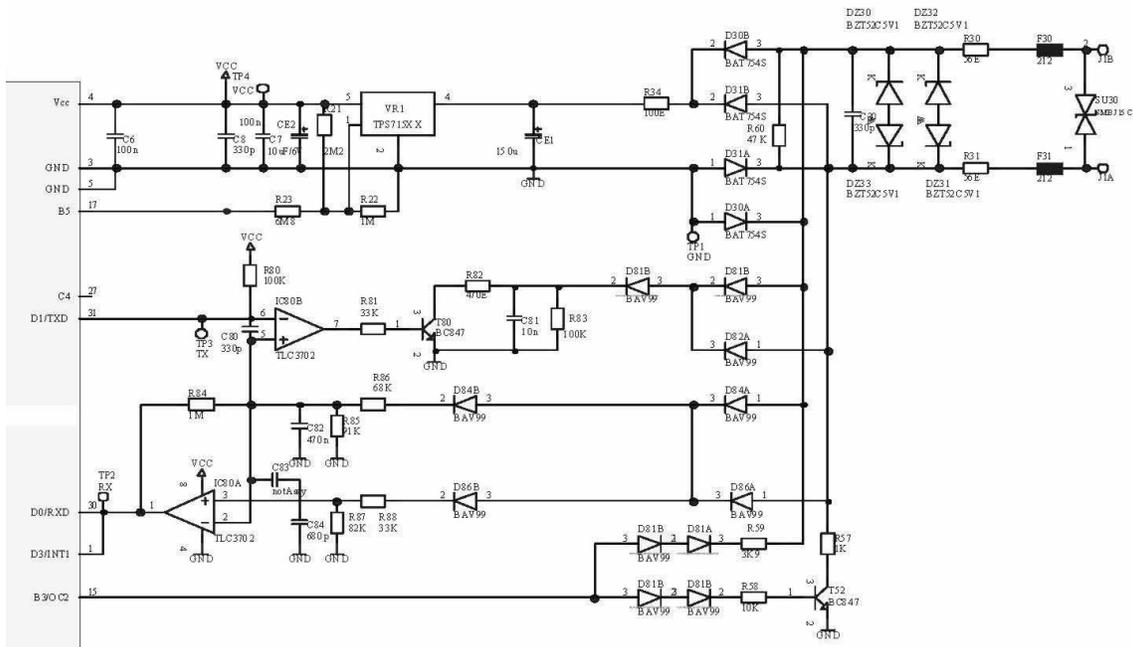
Sample Meter Interface for SCR + for ATEX approval
