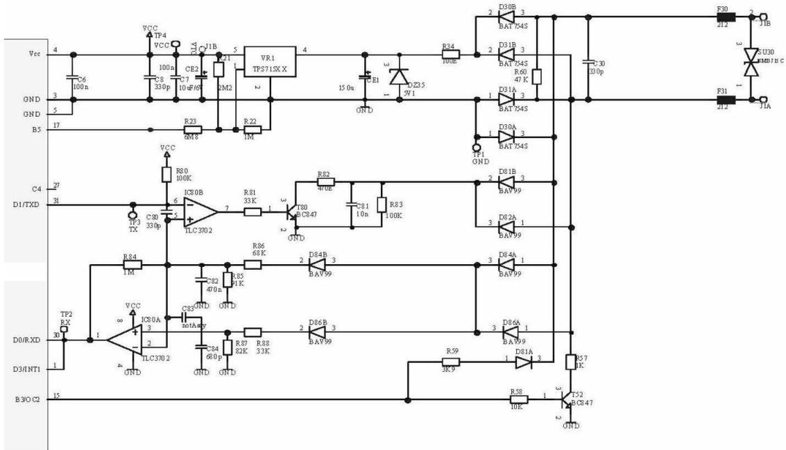
Sample Meter Interface for SCR +
