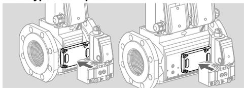
For connecting the bypass/pilot gas valve VAS 1.
