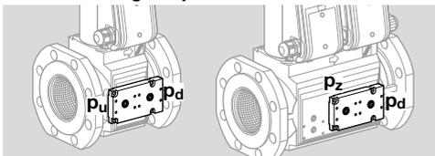
For the connection of the pressure switch DG..C, with a screw plug or pressure test nipple. VAS/VCS 6–9, Order No. 74923021, VAS..T/VCS..T 6–9, Order No. 74923022.
