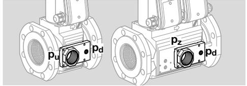
For the connection of a relief line (1½ NPT, Rp 1), with a screw plug or pressure test nipple. Rp 1, VAS/VCS 6–9, Order No. 74923025, 1½ NPT, VAS..T/VCS..T 6–9, Order No. 74923024.
