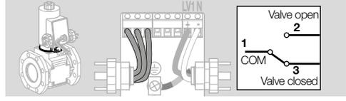
→ Double solenoid valve: if a plug with socket is fitted, only one proof of closure switch can be connected.
