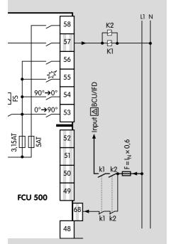
→ BCU with power supply for valves and ignition transformer via safety interlocks (terminal 5)
