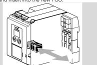
All the parameter settings of the FCU are saved on the parameter chip card.
