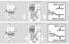
→ When installing two plugs on a VAN with closed position indicator: label the sockets and plugs to avoid confusion.
