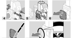
9 Once the seals have been replaced, follow the reverse procedure to reassemble the unit. Note the recommended tightening torques for the connection parts.
