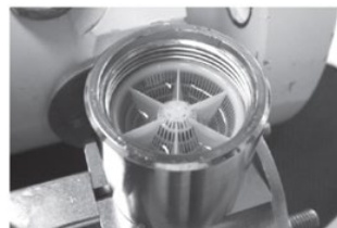
Fig. 5 | Oil supply tank
