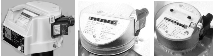
Fig. 3 | Index examples (left: MI-2, centre: S1, right: S1V)
