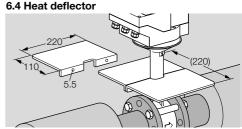
Install heat deflectors in order to protect the actuator from overheating if the medium temperature is > 250°C (482°F).
