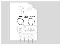
→ Calibration is completed when the blue LED is lit continuously and the red LED goes out.
