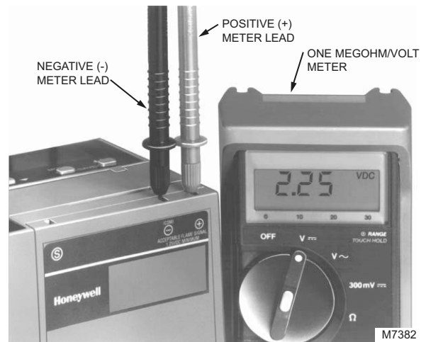
Fig. 17. Flame signal measurement.
