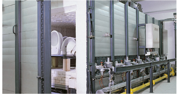
Intermittent shuttle kiln in the ceramics industry
