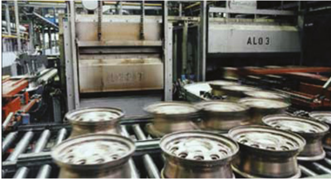
Wheel rim hardening installation
