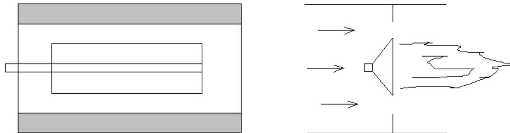
For process air differential pressure drop calculation, use the graphs on the next pages to define the net free area required around the burner. Note that the burner itself creates a displacement area of 185 in.<sup>2</sup> per foot.
