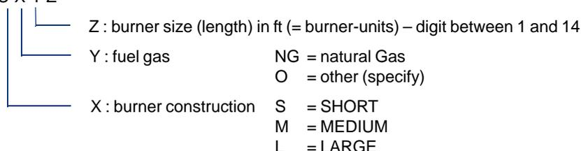
Difference between S, M & L types is because of larger thermal expansion effects on larger burners, requiring special mounting constructions. Since the total duct width is an important factor in selecting the correct burner type, there is some overlapping in the different sizes for some of the burner lengths (see table below).
