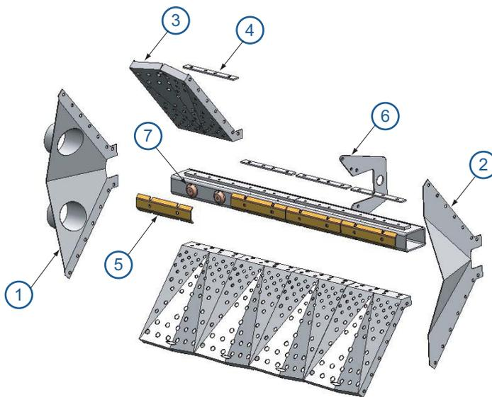
[1] gas nozzles are welded onto the burner manifold and are not available as separate spare parts.
