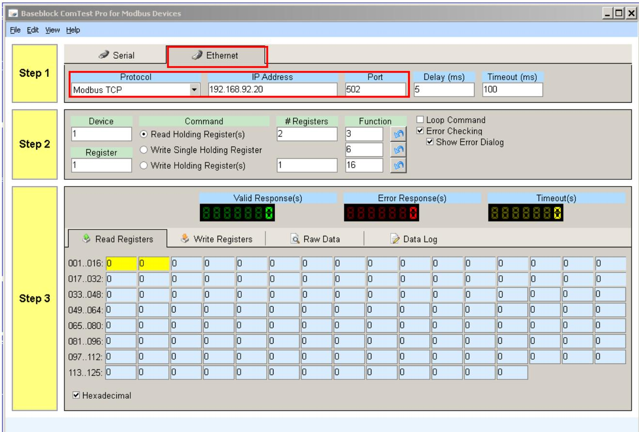
In the initial test we will change the burner set-point from its current value to 150F. If the current value is already 150F, select another set-point value to insure Modbus communication is functioning.
