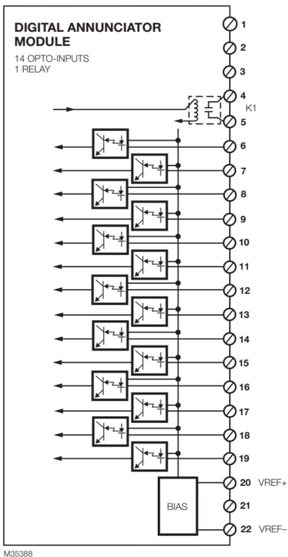
Fig. 4. Annunciator Module terminals.
