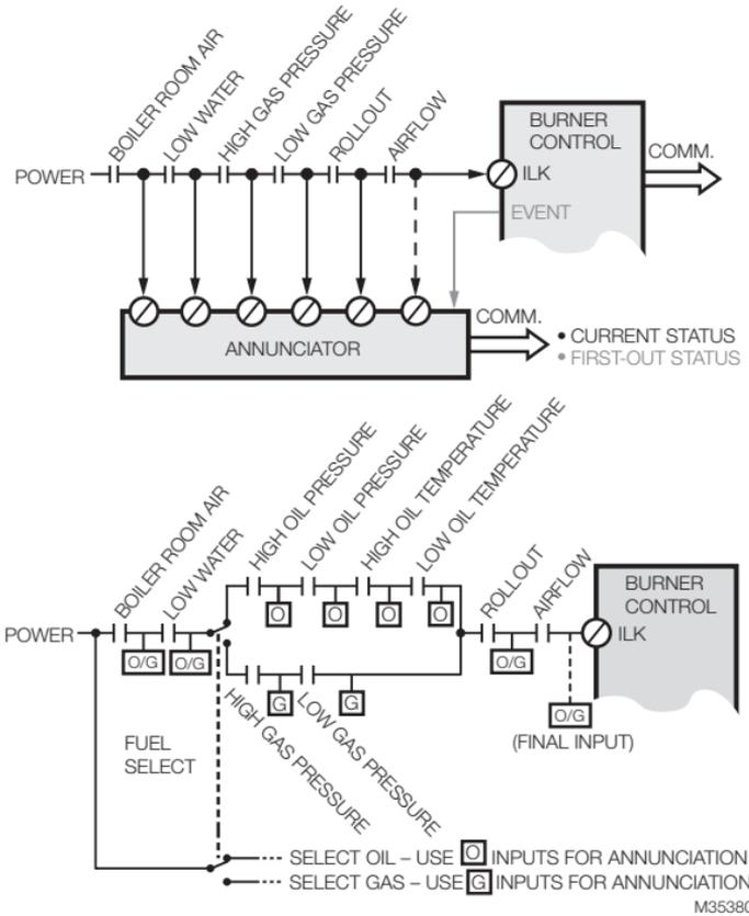
Fig. 3. Wiring diagram for Annunciator Module.
