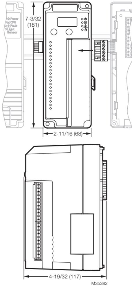
Fig. 1. Dimensions in in. (mm).
