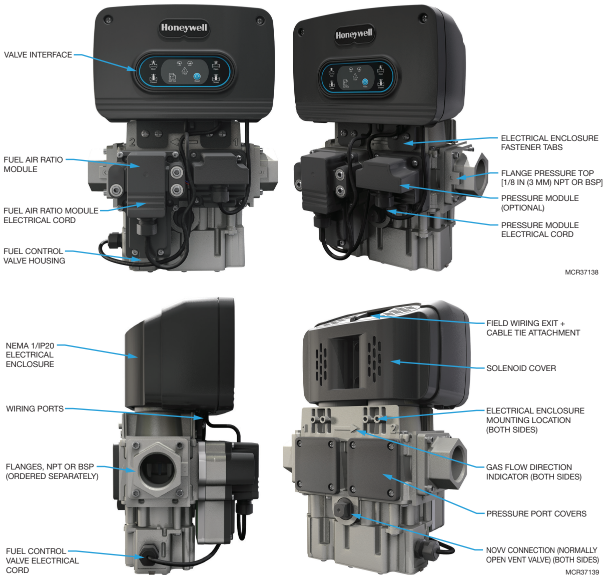
Fig. 13: Valve features.
