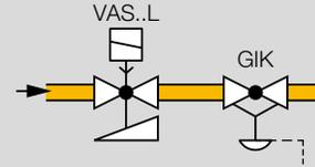
Safety valves must always be installed upstream of the air/gas ratio control GIK. For continuous control, we recommend using slow opening safety valves VAS..L.
