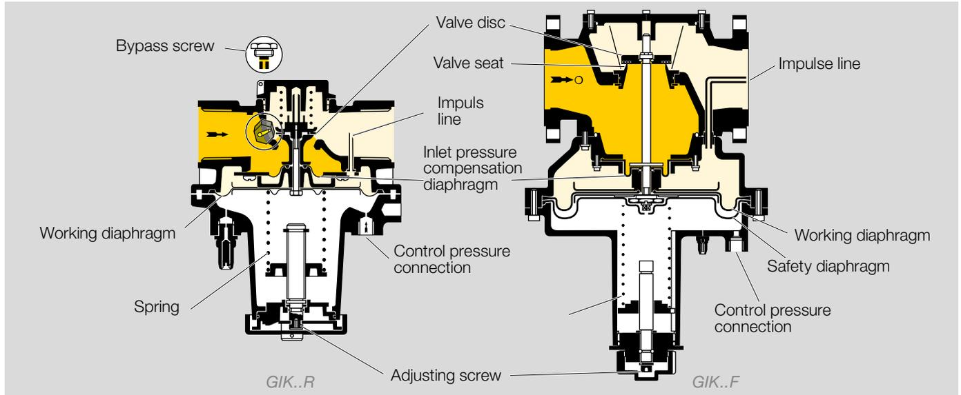
Air/gas ratio control GIK is actuated by the air line pressure. The valve plate is lifted from the valve seat and the gas flows into the regulator outlet area via the open valve seat. The outlet pressure is applied to the space above the working diaphragm via the impulse line. The outlet pressure is controlled in a ratio of 1:1 to the air control pressure. The inlet pressure compensation diaphragm ensures high control accuracy.
