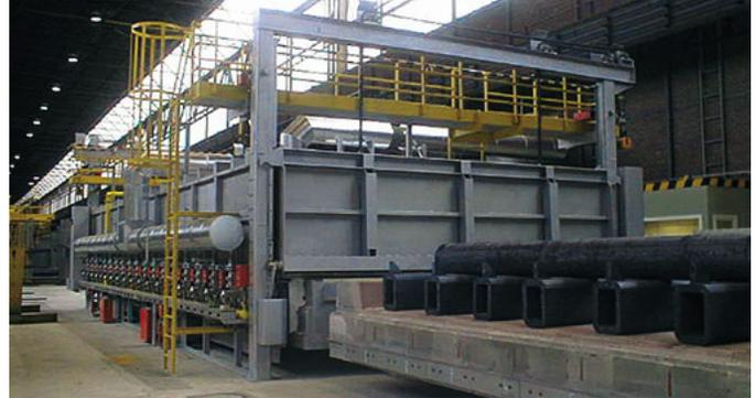
*Metallurgical industry: bogie hearth furnace*
