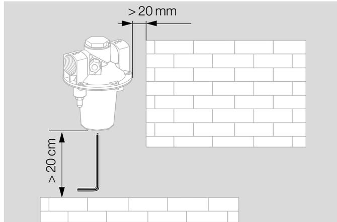
The air/gas ratio control GIK must not be in contact with masonry. Ensure that there is sufficient space for adjusting the low-fire rate.
