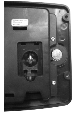
Fig. 6. Install CR2032 coin battery.
