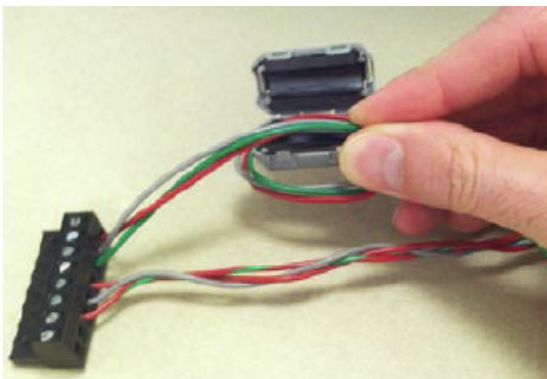
Fig. 3. Install clamp filters on 24VAC and Modbus connections.
