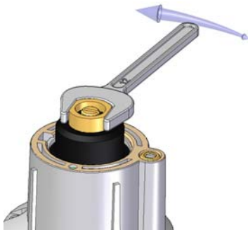
Figure 7 Adjusting flow rate.
