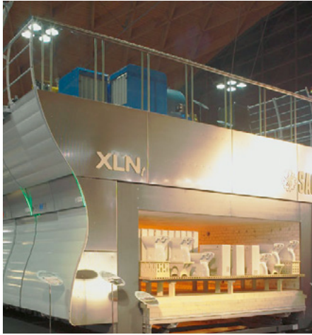
Roller hearth kiln in the ceramics industry
