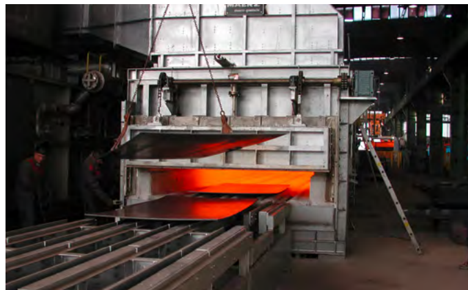
Heat treatment furnace for sheet steel
