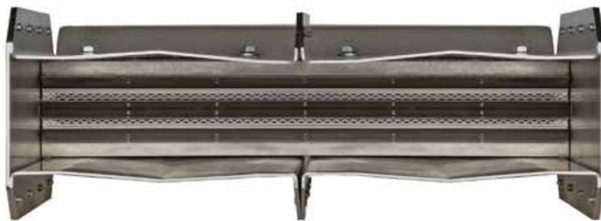
FIGURE 7. Designed in 1' long modules, one ultra-low- \text{NO}_x burner allows for precise heat control and uniformity, making it possible to spread the input of the burner over the whole length of the dryer.
