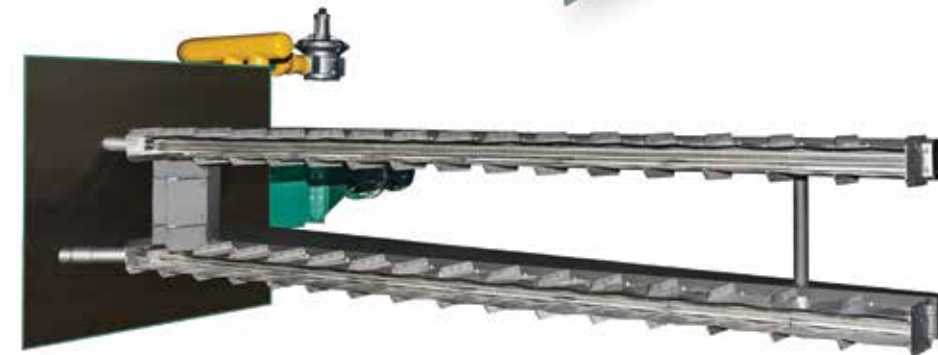
FIGURE 3. An ultra-low- \text{NO}_x burner with seven modules and two rows was designed for a drying application.
