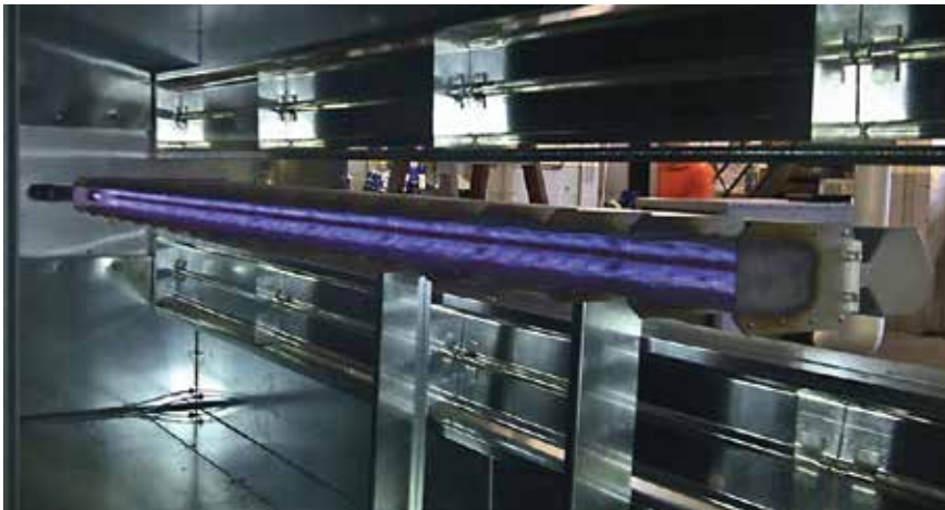
FIGURE 6. The short flame length of the modular ultra-low- \text{NO}_x burner allows it to be used in applications with space constraints.
