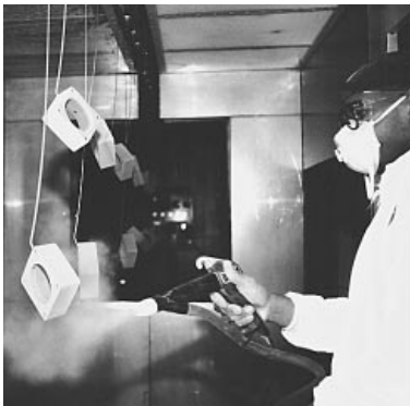
Inside the powder coating booth, parts are sprayed manually by an operator using an electrostatic spray gun. A powder reclamation system gathers and recycles excess powder residue.
