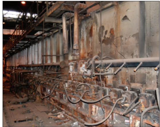
Before: Old Russian U-type burners with radiant tubes and water cooled rollers.
