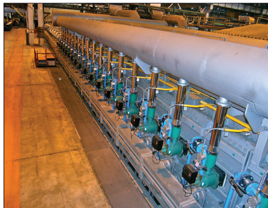
Before: Old Russian U-type burners with radiant tubes and water cooled rollers.
