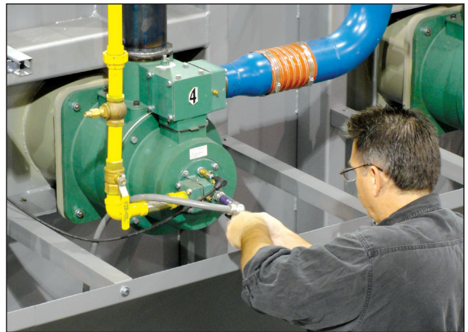
The integrated gas and air orifices and pressure taps are located at the front of the TJSR v5. This feature simplified burner set-up and adjustment during furnace testing.
