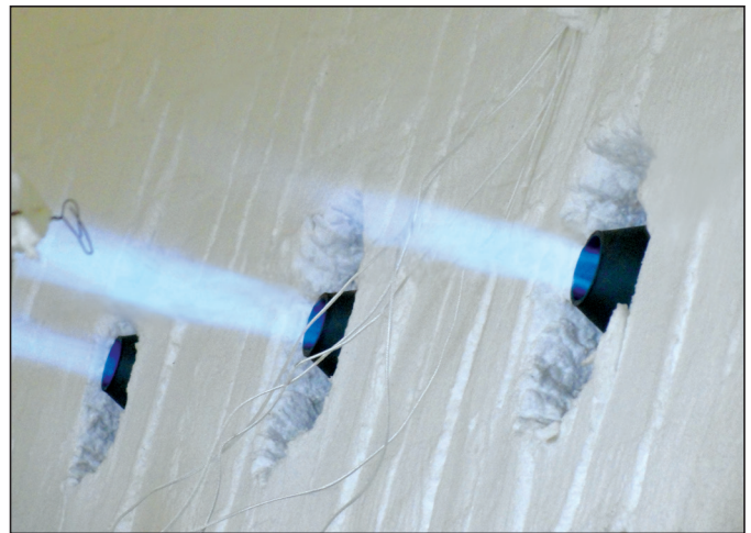
The TJSR v5 delivers a precise, stable flame throughout the full input range. The burner features a high velocity flame along with self-recuperation.
