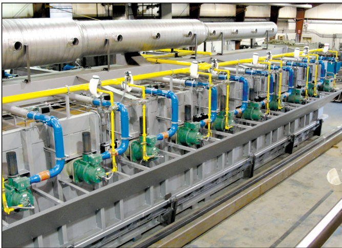
TJSR v5 design eliminates the need for the external hot air ductwork required by other recuperative burners. This provided significant cost savings in the furnace design.
